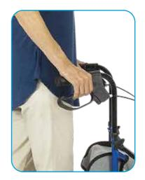
The parking brake is used to help prevent the Rollator from moving when not in use, or to prevent it from moving while sitting or standing. To engage the parking brake, push the parking brake handle down until it locks into a diagonal position, locking it into place. To disengage the parking brake, simply lift up on the handle.
