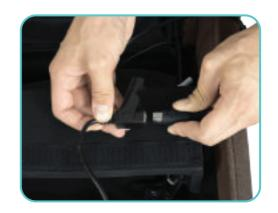
Locate the small black wire on the base of the Frame, and connect the Recliner Transformer wire to it. Insert the Recliner Power Cord into the port on the Transformer, and plug the other end into a power outlet.
