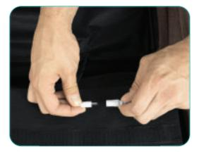
5. Locate the large black wire on the Frame, and attach the Recline/Lift Remote to it to connect the Recliner controls.
