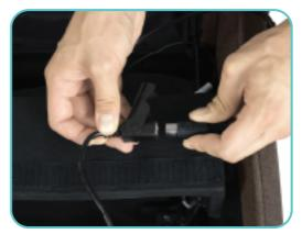
6. Locate the small black wire on the base of the Frame, and connect the Recliner Transformer wire to it. Insert the Recliner Power Cord into the port on the Transformer, and plug the other end into a power outlet.
